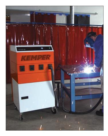
With its four air intakes this mobile extraction and filter unit offers a flexible unit for the extraction of polluted air directly at source.
