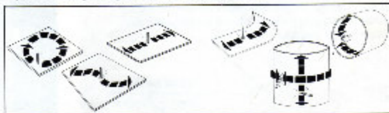
Drive systems and wheel assemblies on Rigid Track (left) and Flex Track Kat Models provide all position welding/cutting capabilities as illustrated below.
