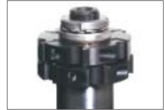
Dual milling heads hold indexable inserts to simplify tool changes while providing a mill quality finish.
