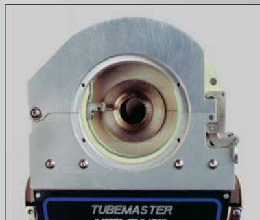
Collets removed to show Fillet Weld
