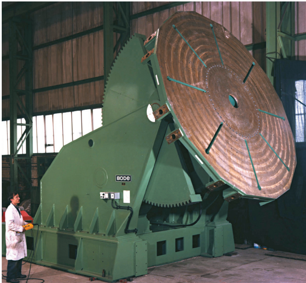
Model VP.100 Special-Positioner (Capacity 100,000 kgs)
