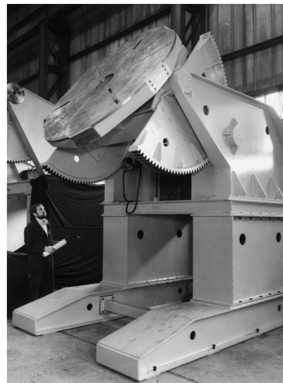
Model VP.20 Positioner (Capacity 20,000 kgs)
