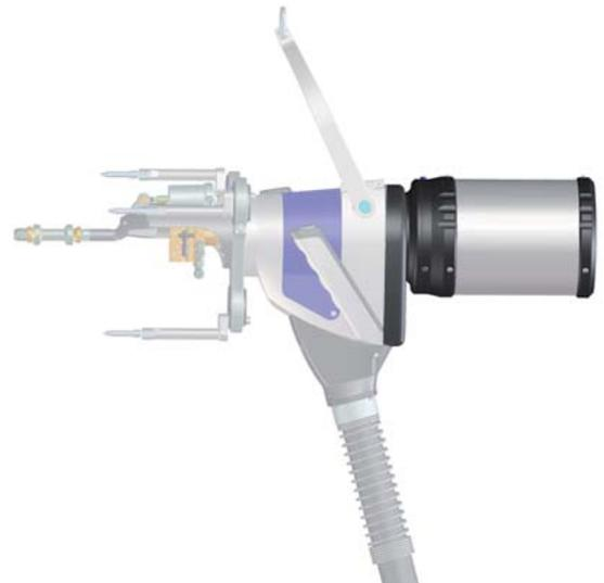
Fig.5.5 - Rotating wire feeder
