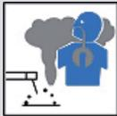
**When welding particularly large parts whose shape creates a confined space or a tank, the operator must make sure that the oxygen content (between 19.5 and 23% of ambient air) is sufficient before intervening. The use of an oxygen analyser is strongly advised.**
