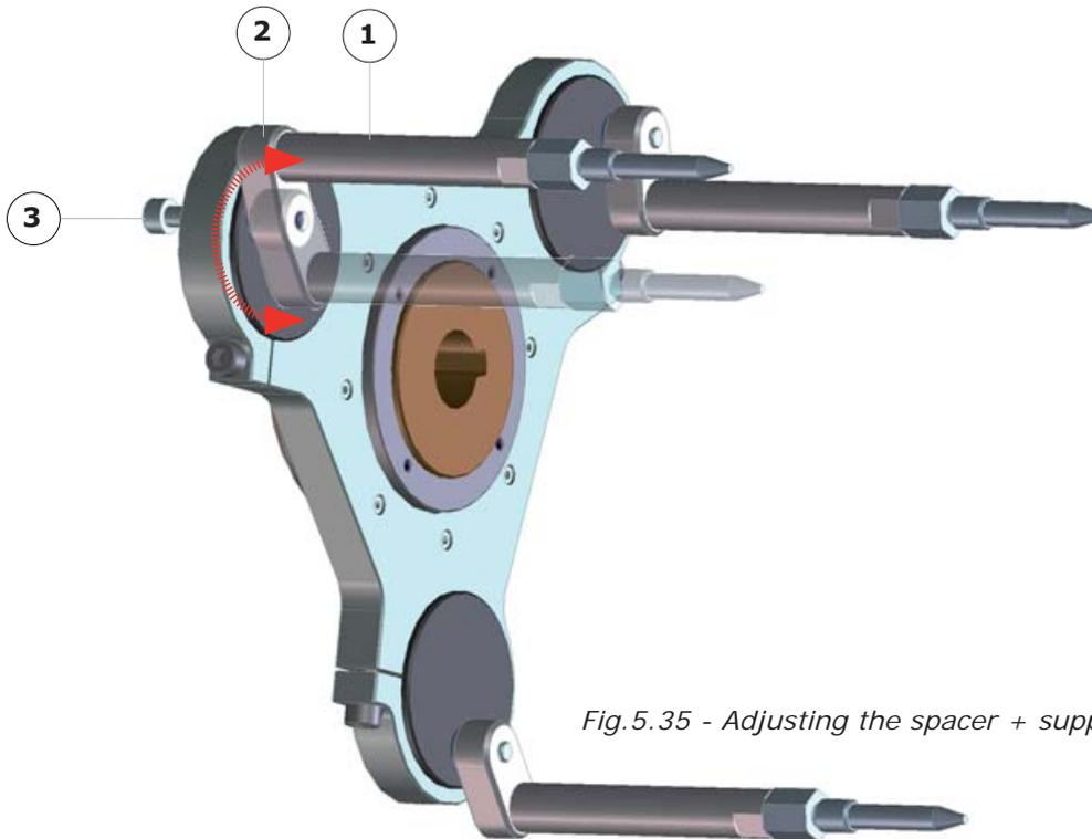
Fig.5.35 - Adjusting the spacer + support leg assembly
