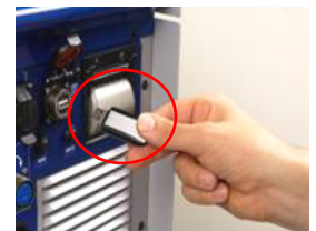
USB memory stick for saving, loading and archiving of welding programs and monitored weld data
