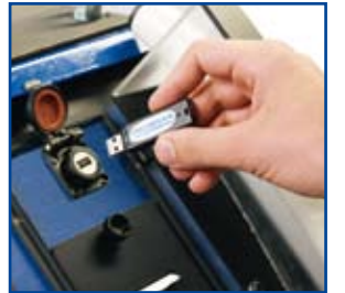
USB memory stick for saving, loading and archiving of welding programs and monitored welding data
