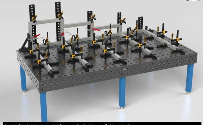
General information: Stops can be firmly fixed or variably adjusted as a result of the combination of oblong slot and system bore holes. Perfect for all flat clamping on the welding table.
