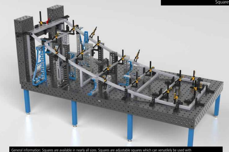
the combination of the system bore holes and the oblong hole. A height-adjustable surface for your welding elements can be created when combining the Stop and Clamping Square with other squares.
