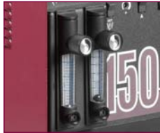
Plasma & Secondary gas flow meter.
