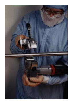
"Compact Design & Ultra Lightweight" allows for easy portability for modification of in-line fabricated tubing.
