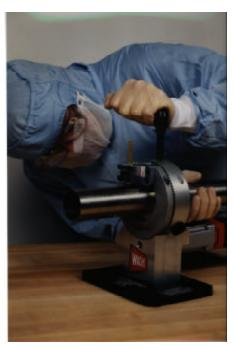
"Clamp Shoe Vise" requires no adjustment for oversize or undersize tubing.
