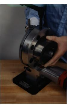
"Quick Change" 300 Stainless Clamp Shoes can be changed from size to size in under one minute.
