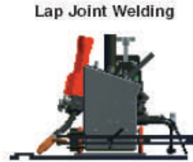
Lap Joint Welding The Moggy is performing a lap joint weld. It is guided by Industry Standard 6" (152.4mm) v-groove Track running parallel to the joint.
