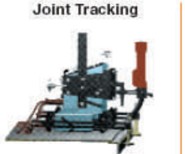
Joint Tracking Adjustable height guide roller assemblies are available to track joints with a vertical member higher or lower than the set height of guide roller wheels.
