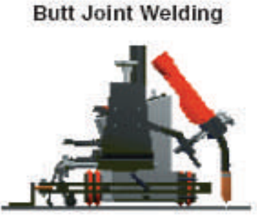
Butt Joint Welding The Moggy is ideal for butt joint welding. Here the Moggy is using a fence to guide it accurately along the desired path. Standard v-groove track can also be used.
