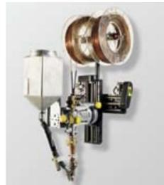
A6S Twin Master for highly productive fillet or butt welding, also on light-gauge material.
