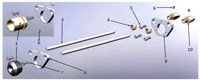
THE STANDARD ASSEMBLIES (SEE TOP OF PAGE) HAVE EITHER THE PIN GUIDE OR THE NOSE CONE (ITEM 1) FITTED. IF BOTH ITEMS ARE REQUIRED THE ADDITIONAL PART MUST BE ORDERED SEPERATELY AS BOTH ITEMS ARE NOT SUPPLIED WITH AN ASSEMBLY AS STANDARD.
