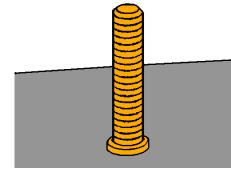
A cold stud weld is noticeable by undercutting of the flange and lack of / minimal formation of spatter. A cold weld is usually caused by too little energy and / or too high spring pressure.
