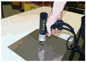
Ensuring that a stud has been loaded, position the stud at the location on the work piece where it is to be welded. Press down firmly on the pistol until all three points of the tripod (or the face of the nose cone if using instead) are firmly in contact with the work piece. Do not drape or wrap the pistol cables over or around yourself whilst operating the equipment. Allow the cables to trail naturally to the floor.
