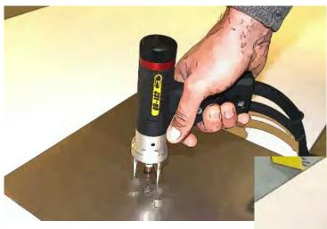
To do this place the pistol into the welding position, pressing down on the pistol until the stud is pressed back into the pistol and all three points of the tripod legs are firmly in contact with the work surface.
