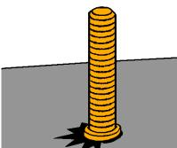
A one sided stud weld (arc blow) is usually caused by incorrect earthing of the work piece. This may be corrected by placing the welding earths opposite each other across the area where the weld is to occur.
