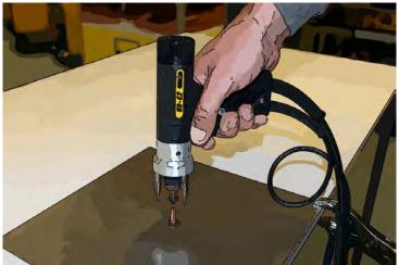
Once welding has taken place. Draw the pistol off the welded stud. Always lift the welding pistol vertically from the welded stud. Failure to do this may cause damage to the chuck, which will result in the chuck and stud arcing together during subsequent welds and thereby reducing the working life of the chuck.
