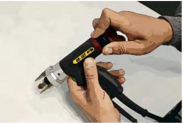
The required lift can now be set. This is achieved by once more turning the rear end cap adjuster in an anti-clockwise direction. The lift adjuster has a click detent which clicks every half turn. Each click (half turn) equates to a 0.5mm change in lift. Therefore a desired
