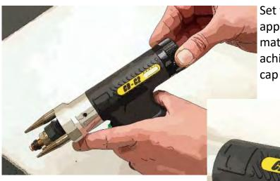
Set the pistol spring pre-load to the appropriate setting for the stud/ material to be welded. This is achieved by twisting the rear end cap adjuster.
