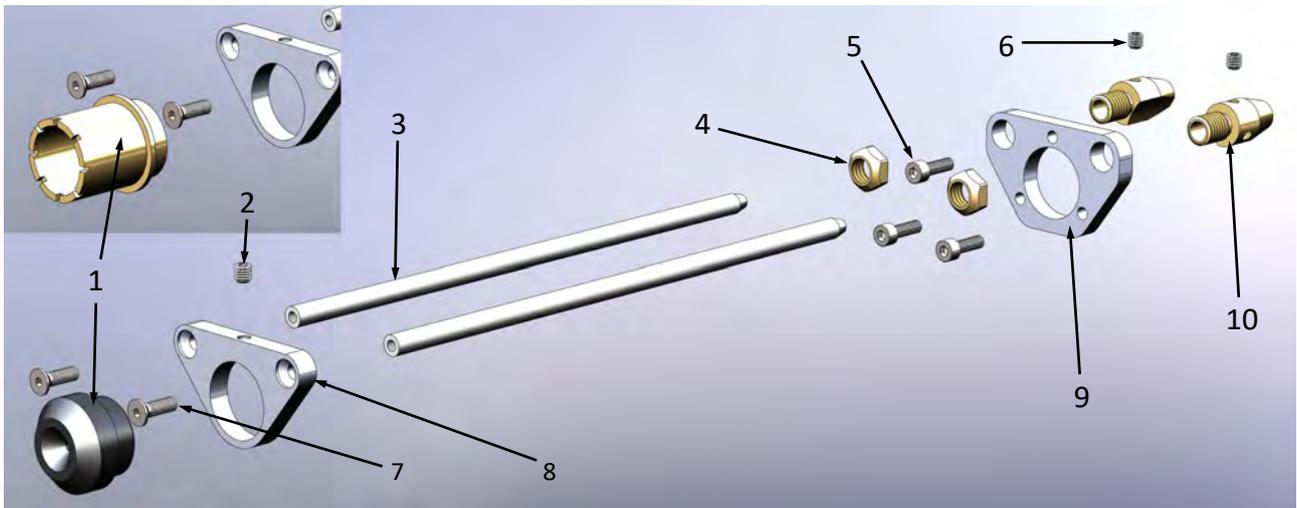
THE STANDARD ASSEMBLIES (SEE TOP OF PAGE) HAVE EITHER THE PIN GUIDE OR THE NOSE CONE (ITEM 1) FITTED. IF BOTH ITEMS ARE REQUIRED THE ADDITIONAL PART MUST BE ORDERED SEPERATELY AS BOTH ITEMS ARE NOT SUPPLIED WITH AN ASSEMBLY AS STANDARD.
