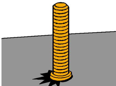
A one sided stud weld (arc blow) is usually caused by incorrect earthing of the work piece. This may be corrected by placing the welding earths opposite each other across the area where the weld is to occur.
