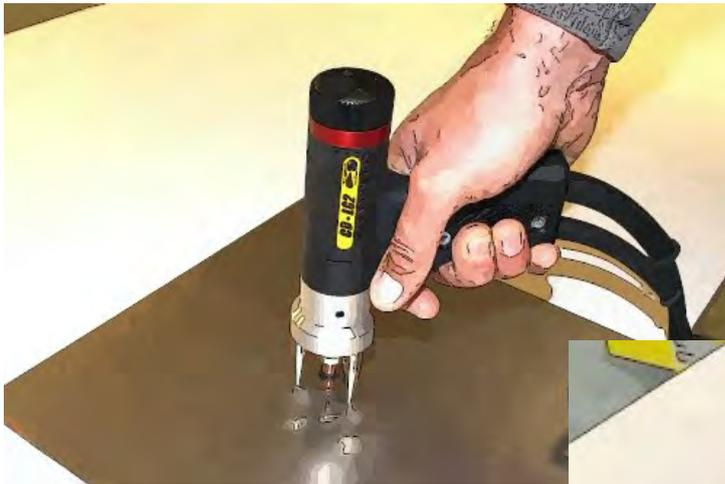
To do this place the pistol into the welding position, pressing down on the pistol until the stud is pressed back into the pistol and all three points of the tripod legs are firmly in contact with the work surface.
