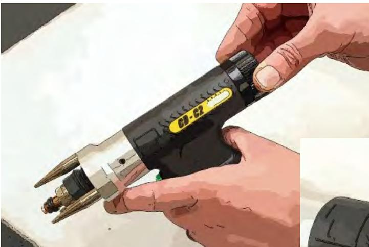
Set the pistol spring pre-load to the appropriate setting for the stud/ material to be welded. This is achieved by twisting the rear end cap adjuster.
