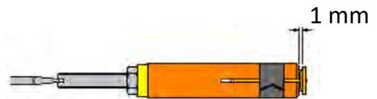
Securely tighten the chuck backstop locking nut to maintain the required protrusion.
