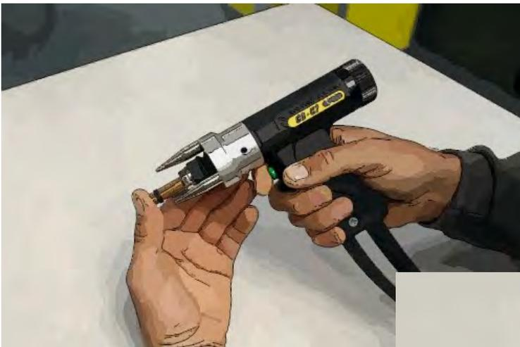
After setting the chuck, insert it into the pistol chuck holder and push firmly home until it comes to a rest.
