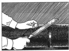
Clean the selected magnet position with a file or wire brush and ensure that the surface is free from oil or grease. Also check that the contact face of the magnet is clean and remove any metallic partials.
