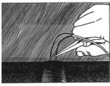
After attaching the thermocouple wire (as described in the OPERATION section) repeat the process for the second wire attaching it 5 or 6 mm from the first wire.
