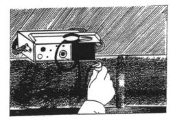
Position the return magnet on the work piece.
