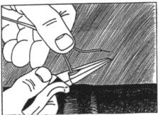
Using the supplied pliers, pull back the insulation at the end of each wire to give 10 mm of bare wire.
