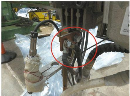
1 x Flex Armoured cable multicore – 4 wires used connected to transformer in Esab unit. Terminal block marked with wire numbers
