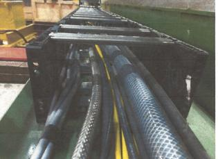
Most of the cables in the cable tray were unused and not connected to anything. These were removed from the cable tray and place in the packing tray with the other parts.
