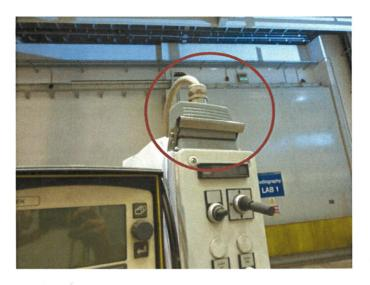
1 x Purple cable that connected the PEK control box. This cable has two solder connections to a small circuit board located at the top rear of the control box. The circuit board has two external sockets. The wires were snipped to show were the cables connected.
