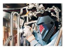
variable high frequency PULSE facility is included. This unique feature allows the arc to be adapted to suit the application while reducing heat input. The result being a more controlled weld, less distortion and increased welding speed. Development focused further on the needs of the welder by designing the control panel to illustrate the welding se-quence, making it user friendly, clear and easy to understand.
