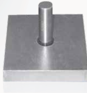
12 mm hole cutting without True Hole Technology
