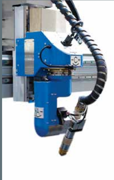
Can move totally 180 degrees at A axis.
