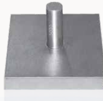
12 mm hole cuts with True Hole Technology
