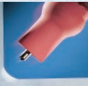
Cap diameter: 3.2 mm Base metal: AlMg3 Sheet thickness: 5 mm Welding current: 185 A Welding voltage: 15.6 V AC Balance: 0
