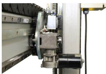
Boom movement with rack and pinion
