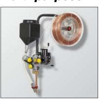
SAW is one of main features of the A2-system. The pro-ductivity and quality can be improved considerably by using a welding head with a twin wire kit (double wire).
