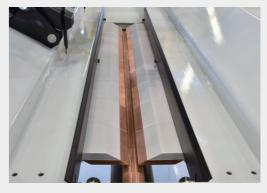
Finger clamp is constructed with two materials - copper and aluminum
