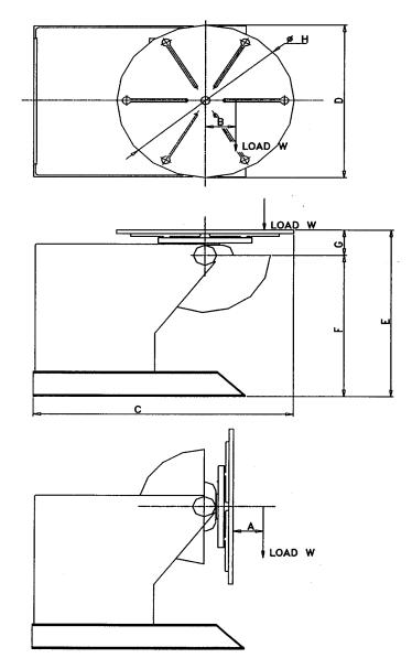
ROTATION TORQUE (R) IS A STRAIGHT FORWARD CALCULATION OF LOAD (W) X ECCENTRICITY (B) BUT TO ENSURE AN ACCURATE FIGURE FOR TILT TORQUE (T) IT IS IMPORTANT TO USE THE FULL DISTANCE TO THE PIVOT POINT. THIS IS OBTAINED BY ADDING TOGETHER THE CENTRE OF GRAVITY (A) AND TABLE PIVOT DISTANCE (G). THEREFORE :- ROTATION TORQUE (R) = W X B Kg METRES TILT TORQUE (T) = W X (A + G) Kg METRES MULTIPLY BY 9.81.
