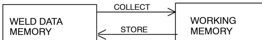
The working memory is used to store a complete set of welding parameters, which can then be saved in the weld data memory.
