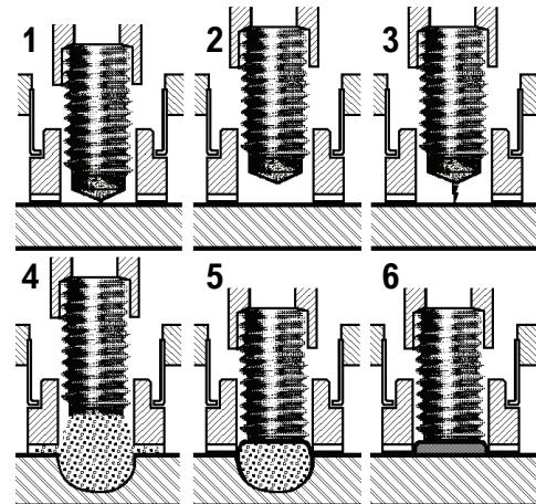
Having welded the stud, draw the pistol vertically off the stud. Failure to do this may cause the split tines of the chuck to splay out. This will result in the chuck and stud arcing together during subsequent welds.
