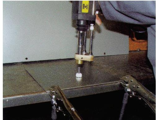
Finally, remove the ferrule by lightly tapping until it shatters. Visually inspect the weld.
