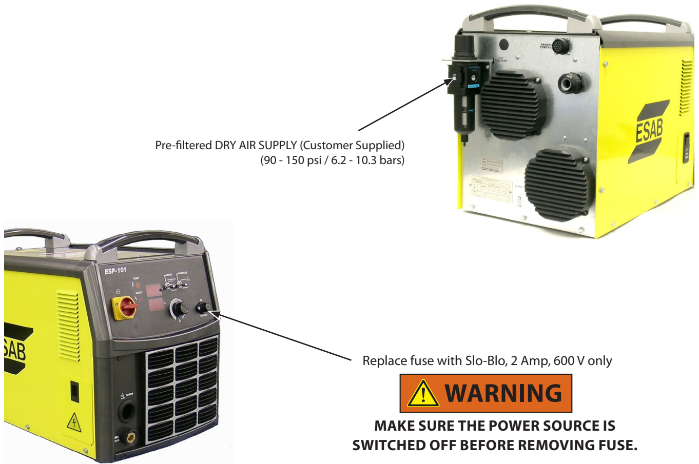
Figure 3-4. Input Connections / Fuse Replacement
