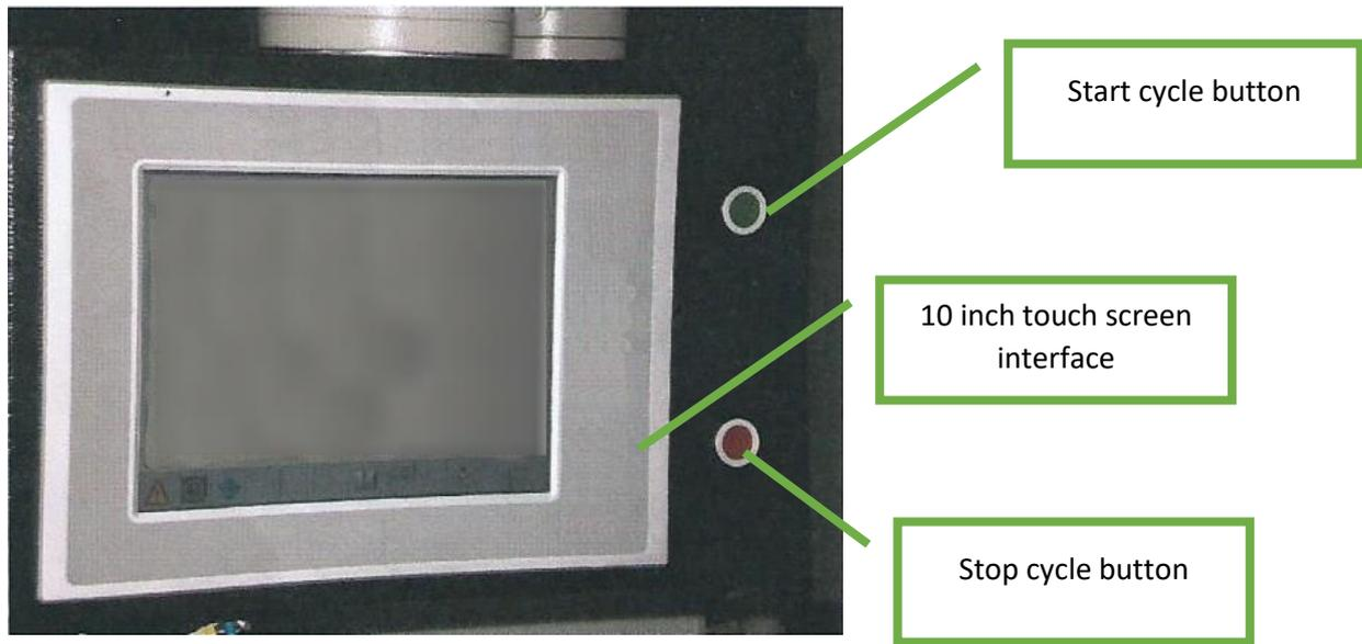
Figure 1 operators console front view
