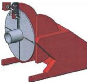
During welding the turntable rotates and the X axis moves along the length of the cylinder at each offset.
