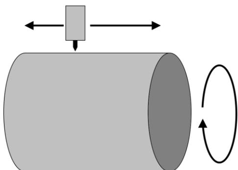
On initial start up of the weld the position of the AVC axis (in millimetres) is measured. Subsequent changes in the position of the AVC axis result in a recalculation of the work piece diameter. This allows for the changes in diameter due to layering or tapered work pieces.
