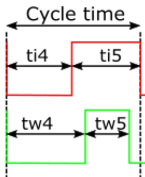
This allows the wire to be started and stopped earlier or later than the peak welding current to optimise the wire feed.
