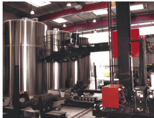
Standard turntable 5 to 30 T Up to 4500 mm diameter
