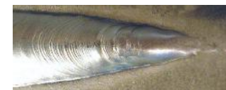
Excellent weld finishing
