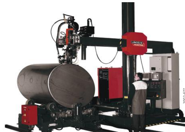
Elliptical welding with column and boom on rotator
