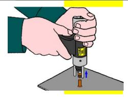
Visually inspect the weld. A good weld will result in an all round weld with a small visible witness of spatter surrounding the flange of the stud.
