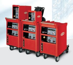
/ VarioSynergic is a microprocessor-controlled MIG/MAG welding system consisting of a power source, a wirefeeder, a welding torch and a cooling unit. Synergic Mode makes the system much easier to handle: just set the sheet thickness and the filler metal, and leave the power source to adjust everything else by itself. VarioSynergic is available in two different versions: a compact version with an integral wirefeeder, or with an external wirefeeder for portable deployment.
