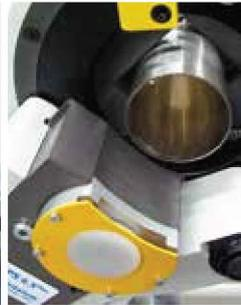
Tried-and-tested planetary cutting technology: The saw blade immerses into the cut and is guided orbitally around the tube
