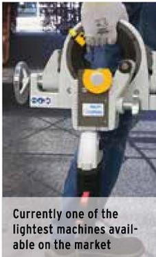
Deformation-free clamping of thin-walled tubes
