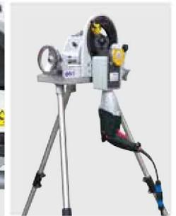
Tripod made of aluminum optional available. Can be dismantled in a few steps - for space-saving storage, for example in the PS transport case
