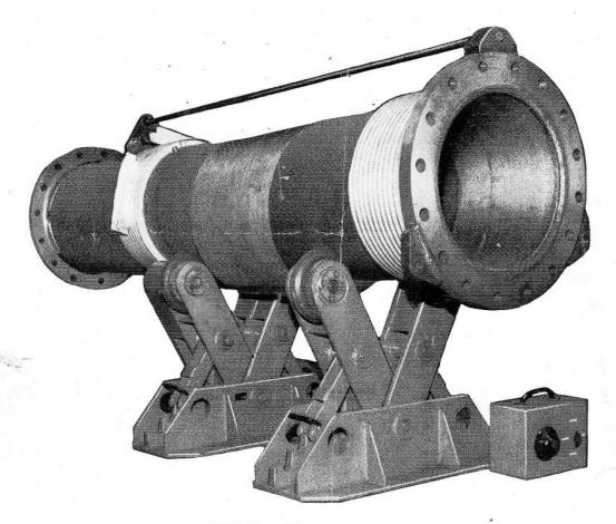
1/CR 40 'SIZZER' ROTATORS 2 tons capacity. (By courtesy of Sheetfabs Ltd.)
