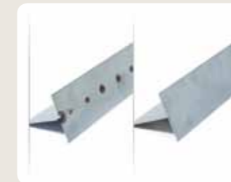
The difference in the tack welds is clearly visible. MicroTack was used to weld the piece on the right, and usual TIG was used on the piece on the left.
