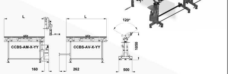
The system is delivered with the height-ajustable support bench (CCBSB-X1), additionnal support benches, the starting end stop module and its extensions.
