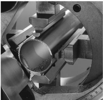
The precision of our cutting machine allow a perfect tube to tube alignment with the smallest gap possible, removing the need to facing the tube therefore saving a significant amount of time and money.
