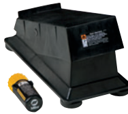
Wireless Remote Foot Control #300 429 For remote current and contactor control. Receiver plugs directly into the 14-pin receptacle of Miller machine. 90-foot (27.4 m) operating range.
