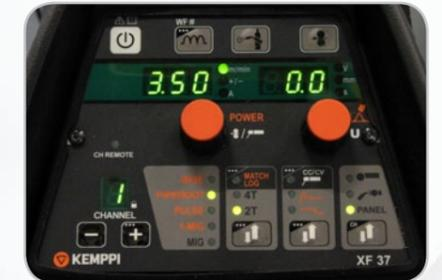
XF 37 control panel of the MXP 37 Pipe wire feeder.
