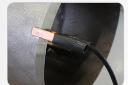
Voltage sensing cable measures the actual arc voltage during welding. This allows PipeRoot to optimise welding characteristics, which results in low-spatter filler material transfer and a stable welding arc.
