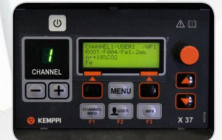
X 37 control panel of the FastMig X 450 power source.
