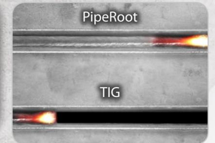
PipeRoot takes you 5 times further in root welding compared with TIG process. No backing needed, good quality, less grinding and preparation work.
