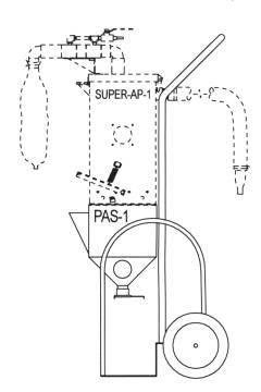
PAS-1/SUPER-AP-1 comes complete with with 15 feet of 1-1/2" hose and flux pick-up nozzle.
