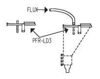
The PFR-LD3 Lid is for attachment to most manufacturer's standard flux hoppers (please specify model of hopper used when ordering), to pressure feed flux to the hopper from a flux feed pressure tank (PT-"x"00, HPT-"x"00, PFR-3 and LPFR-3 systems). Customer has choice of 1/2", 3/4" or 1" I.D. hose fitting.
