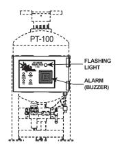
High or low flux level warning lights or audible alarm for flux level. (Consult factory if high and low flux level sensing is required.)
