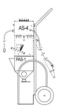
PAS-1/AS-4 comes complete with 15 feet of 1-1/2" hose and flux pick-up nozzle.
