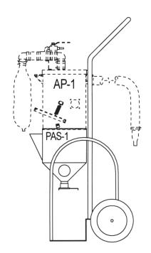
PAS-1/AP-1 comes complete with 10 feet of 1-1/2" hose and flux pick-up nozzle.
