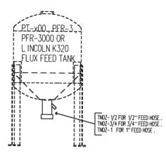
1. **TNOZ-1/2"** - Pressure tank flux feed nozzle for 1/2" I.D. hose. Nozzle fits 2" NPT female pipe fitting which is standard on PFR-3, PT-"x"00, HPT-"x"00, PFR-3000, and Lincoln K320 tanks.
