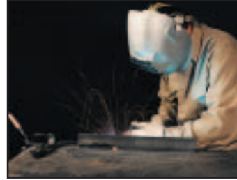
STT using CO 2 and .045" solid wire. Note reduced spatter and fume.
