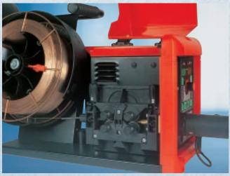
4-roller drive for precision, abrasion-free wirefeed.
