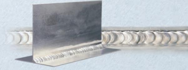
Base metal: AIMg 3 Sheet thickness: 0.6 mm Filler metal: AIMg 5, diam. 1.2 mm Shielding gas: Argon
