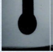
Conventional power source: End of welding without burnback impulse.
