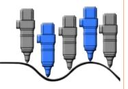
**Height Automatic Adjustment System.** Non-contact height following function; Adjusting the focal length precisely and automatically according to the height of metal plate.
