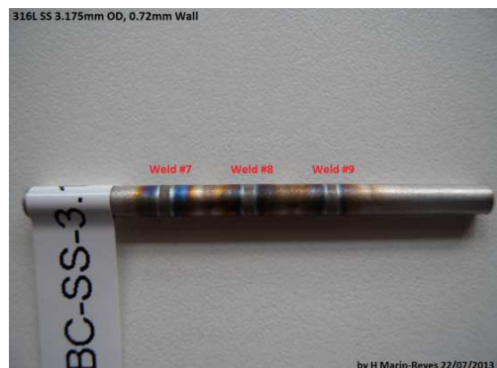
Figure. (a) Welds #7 to #9 on 3.175mm OD, 0.72mm wall 316L SS tube
