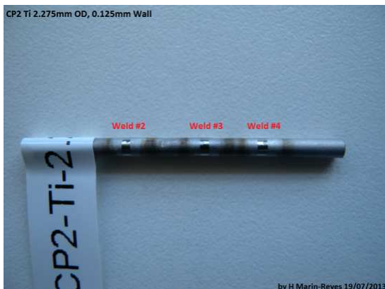
Figure. (a) Welds #2 to #4 on 2.275mm OD, 0.125mm wall CP2 Ti tube
