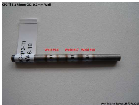
Figure. Welds #16 to #18 on 3.175mm OD, 0.2mm wall CP2 Ti tube
