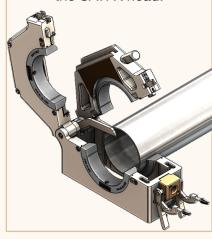
Interface to be fixed on the welding head.
