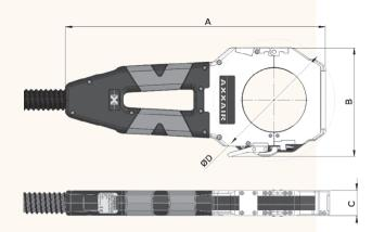
Thickness of 37.6 mm: possibility to weld with the stainless steel jaws standard microfitting fittings or other accessories with a straight part of 19.1 mm.
