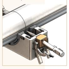
The cassettes benefit from the same closing system with adjustable force without tools that allows precise adjustment of the jaw force on the tube to be welded and assists opening after welding.
