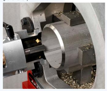
Above a thickness of 3 mm, simple fusion involves a melt volume that is too significant to guarantee proper geometric control of the weld bead. To remedy this, bevelling reduces the quantity of material to be fused in order to achieve proper penetration.
