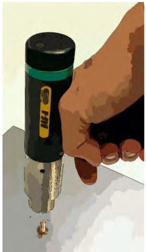
Once welding has taken place. Draw the pistol off the welded stud. Always lift the welding pistol vertically from the welded stud. Failure to do this may cause damage to the chuck, which will result in the chuck and stud arcing together during subsequent welds and thereby reducing the working life of the chuck.
