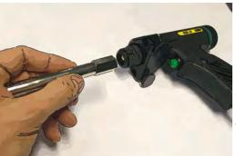
Slide the chuck into bellows support and screw the chuck into position on the M10 mounting thread on the front of the pistol shaft.
