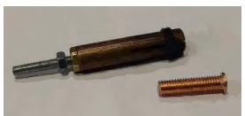
to a maximum length of 40mm). This is because the pistol variants using the CD type chucks have a fixed length setup. The stud must be inserted fully into the chuck until the flange of the stud hits the face of the chuck and then adjusted out by turning the adjuster screw until there is an approximate gap of 3 - 4mm between the face of the chuck and the
