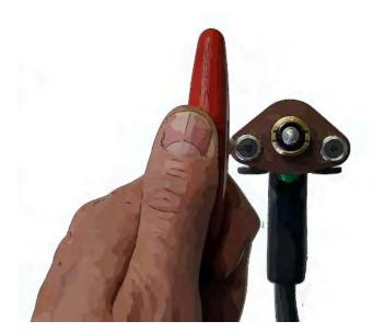
Remove the ferrule and check the centrality of the stud in the ferrule grip by looking straight down the centre of the pistol shaft. If the stud appears to be off-centre. Use a 3mm hex key to loosen the foot screws on the foot adaptor and re-position the adaptor on the legs (the holes in the adaptor are designed to allow adjustment). Re-tighten the screws once the adjustment has been made.
