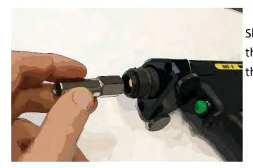
Tighten the chuck into position using an appropriate wrench (usually 14mm A/F for Euro chucks - see page 25).
