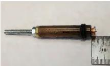
CD type chucks have an adjustable backstop which needs to be adjusted to suit whatever length of stud has been selected (up
