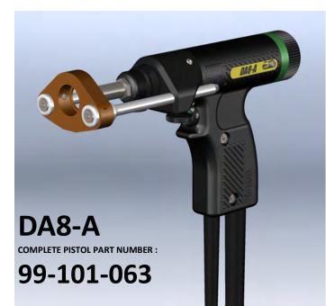
The basic standard model of the DA8-A pistol is shown here on the left. This model is supplied rigged as standard to use European screw-on chucks and for welding standard drawn arc studs with ceramic ferrules .
