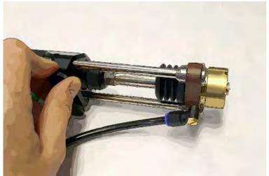
Check the centrality of the stud in the nose cone by looking straight down the centre of the pistol shaft. If the stud appears to be off-centre. Use a 3mm hex key to loosen the foot screws on the foot adaptor and re-position the adaptor on the legs (the holes in the adaptor are designed to allow adjustment). Re-tighten the screws once the adjustment has been made.
