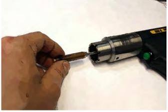
IMPORTANT! Do not over-tighten chucks. This requires only hand tightening. Over-tightening may result in un-warrantied damage to your pistol.
