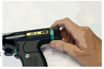
Stage two is to "zero" the lift. NOTE Ensure that the pistol is not connected to the
