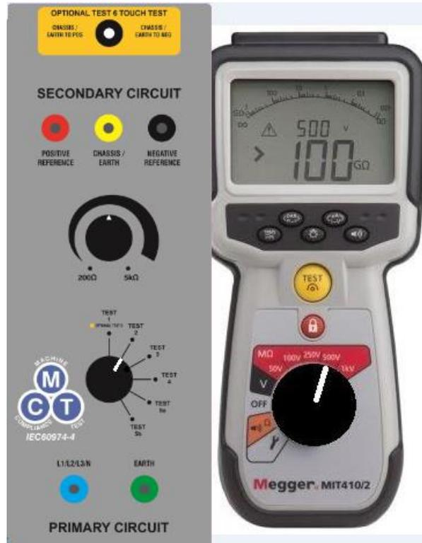
Select switch position 2 on the MCT Unit. Turn the Megger to the 500v position. Press and hold the test button and record the result in the box and press enter.
