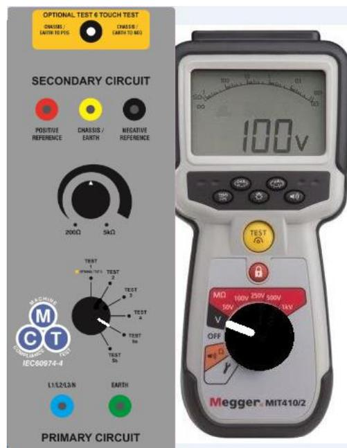
Turn the output of the welder on taking care to disable or disconnect HF which could damage the Megger and ensure any Voltage Reduction Device (VRD) is turned off. If it is impossible to turn off the VRD then record the low voltage and during the function test ensure the VRD is operating correctly. NB – if you do not see a voltage reading double check you have the polarities the correct way around.
