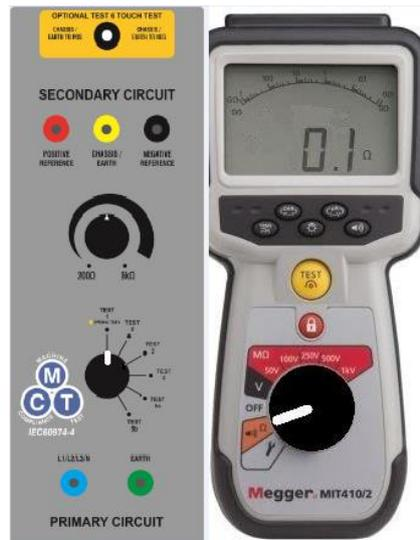
During the measurement, the cables shall be bent, flexed or twisted along the whole length, Especially in the vicinity of cable entries into the enclosure, in order to detect interruptions in the protective conductor. This will highlight any breaks / defects.
