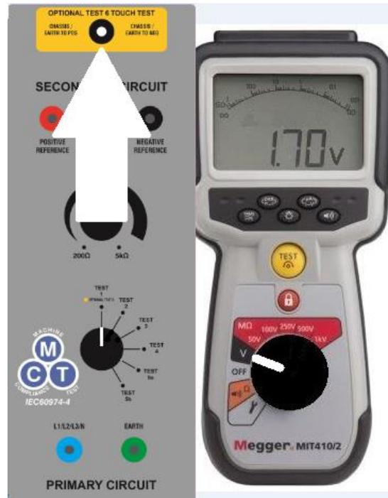
Turn the output on with the Positive, Negative and Chassis leads connected. Push the touch test switch to the Positive – earth position. Take the voltage reading from the Megger and insert into test box 6a. For example – as above enter 1.70, this equates to 1.70mA when Ohms law is applied. If the reading was 22.4 volts we would enter 22.4 in the box. That would equate to 22.4mA and a fail situation.
