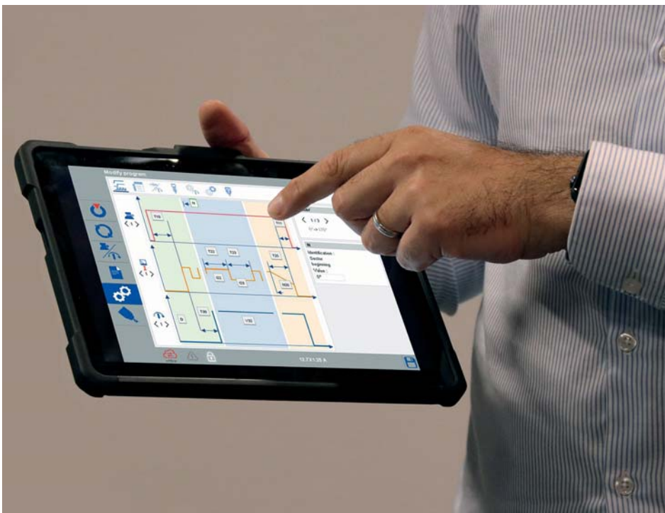
Figure 3. Wireless touchscreen controller to pilot one or several welding installations.
