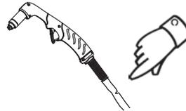
Inspect the torch lead. Replace if damaged.
