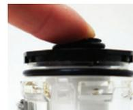
**Install the air filter element (for guarded metal bowl)**
