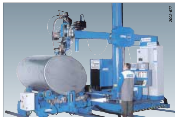
Elliptical welding with column and boom on rotator.
