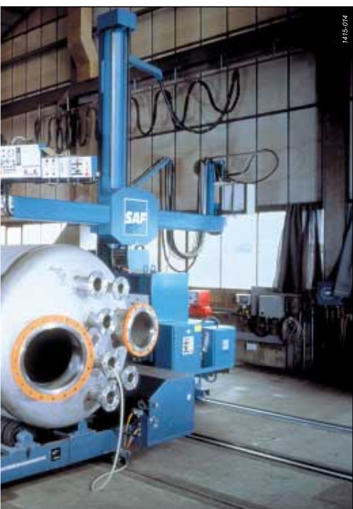
Elliptical welding with column and boom on rotator.
