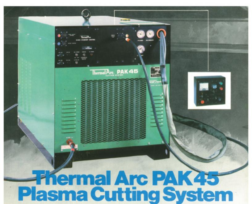
The PAK 45 is a compact, versatile plasma cutting system designed for high speed cutting of most metals up to 2" thick (51 mm), with maximum cutting capability to 3" (76 mm). The cutting current is continuously adjustable between 50 and 400 amperes, to enable quality hand or machine cutting over a wide range of material thicknesses.
